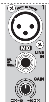
Fig. 2.1: Connectors and controls of mic/line inputs
